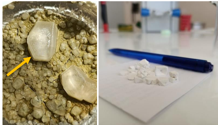
Fig. 8. Picture of boron crystals formed in the beaker after sonication (a) and the boron crystals separated from clays (b)
