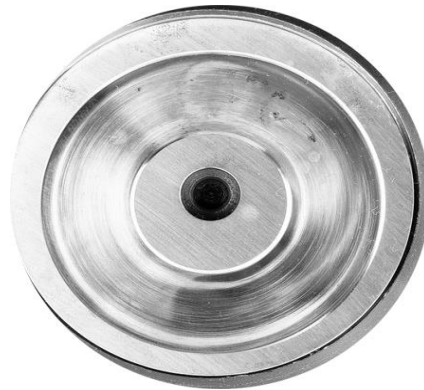
Figure 2. Demonstration of deflected swashplate wear
