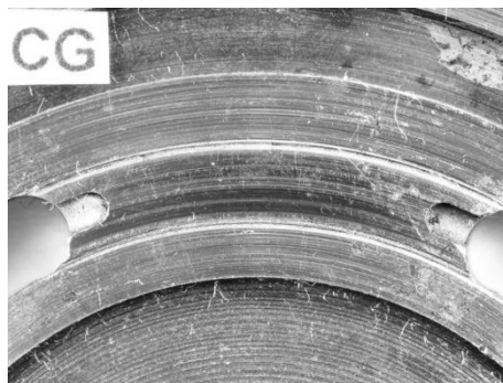
Figure 3. View of flow micro-conduits on worn valve plate
