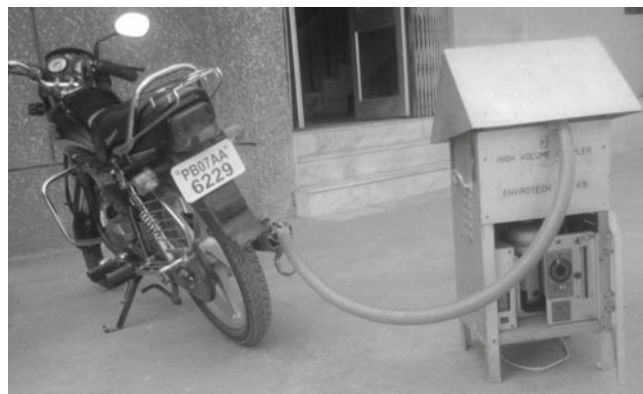
Figure 1a. Sampling of two wheeler exhaust (on standing mode) through high volume sampler
