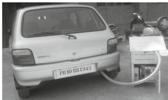
Figure 1b. Sampling of the four wheeler exhaust (on standing mode) through high volume sampler
