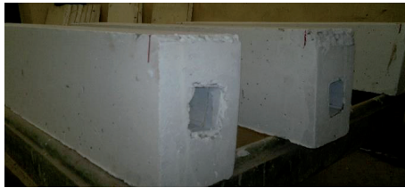
Fig. 6. HLC Beams out of the Water
