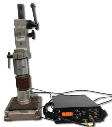
Fig. 3. Research set-up for ultrasound tests of pathways of bonding moulding sands with chemical binders
