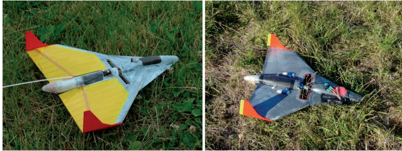
Fig. 4. First flying prototype of the MAV on the left, second prototype on the right
