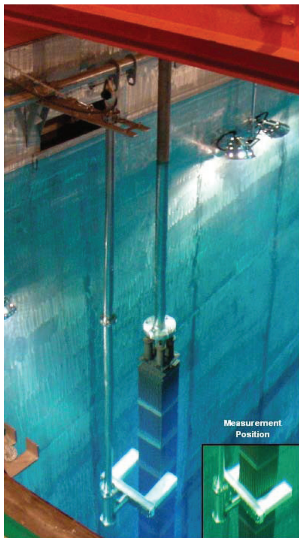
Fot. 3. Pomiar wypalonego paliwa Fork Detector Photo 3. Fork detector irradiated fuel measuring system - FDET) (IAEA)
