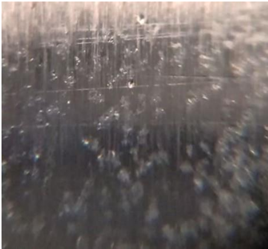
Fig. 13. Photo of the contact surfaces (magnification \times 240 ). Test 3: v=220 cSt; V=1600 rpm; T=125 \mu\text{m} ; Q=160 N
