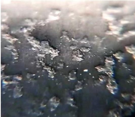
Fig. 12. Photo of the contact surfaces (magnification \times 240 ). Test 2: v=220 cSt; V=800 rpm; T=90 \mu\text{m} ; Q=130 N
