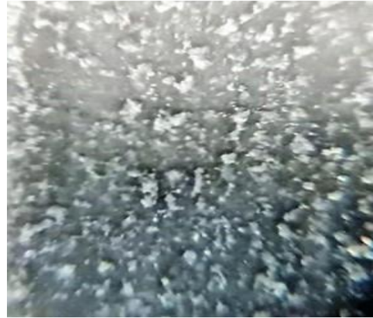
Fig. 15. Photo of the contact surfaces (magnification \times 240 ). Test 5: v=150 cSt; V=200 rpm; T=90 \mu\text{m} ; Q=160 N
