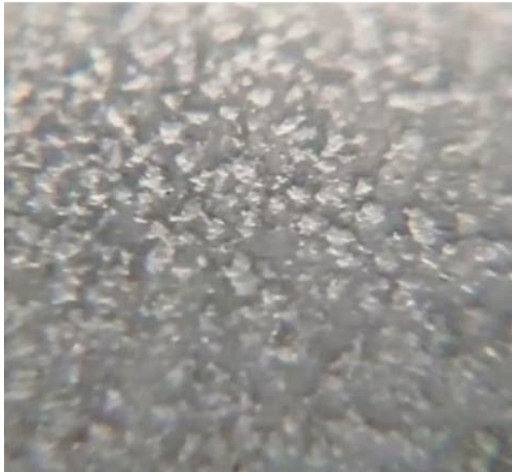
Fig. 19. Photo of the contact surfaces (magnification \times 240 ). Test 9: v=37 cSt; V=200 rpm; T=125 \mu\text{m} ; Q=130 N.
