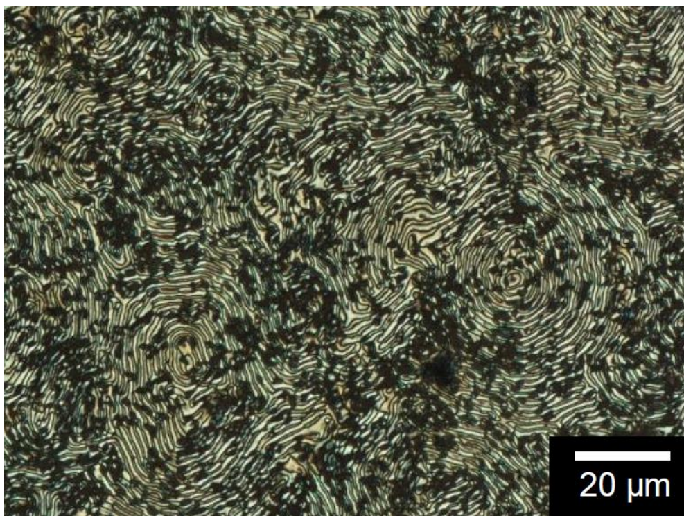
Figure 3. Polarising optical microscopy image of a polymer thin film prepared in cholesteric liquid crystal electrolyte solution.
