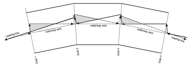
Figure 6. Schematic diagram of navigation in leading lines in the opposite directions
