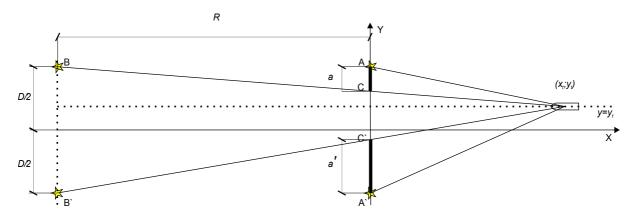
Figure 3. The use of Thales assertion in the description of a rectangular leading line in a Cartesian coordinate system
