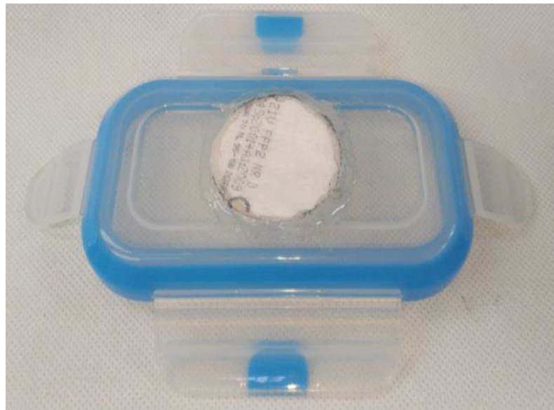
Fig. 7. A fragment of mask filter glued to the cover of the hermetic box before its testing
