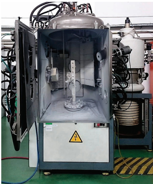
Fig. 1. The technological equipment and scheme of surface treatment technology: a) MZ383 device, and b) the scheme of Arc-PVD technology
