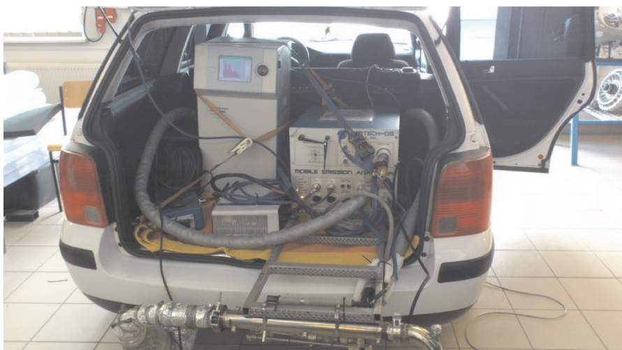
Fig. 3. PEMS measuring equipment during installation inside the vehicle
