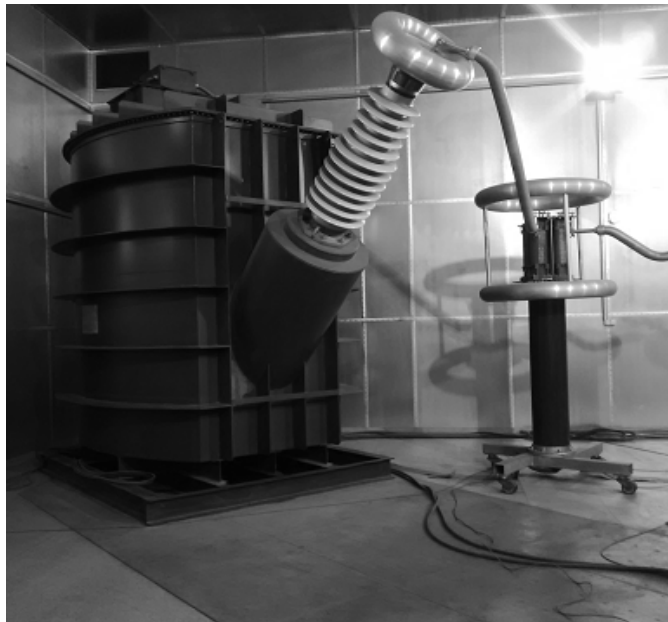
Fig. 3. Resonant Test System RS-700-30-50 made by Haefely Trench
