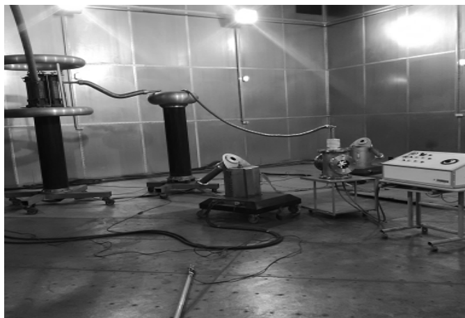
Fig. 4. Stand for measuring the acoustic emission and the dielectric strength of the insulation system
