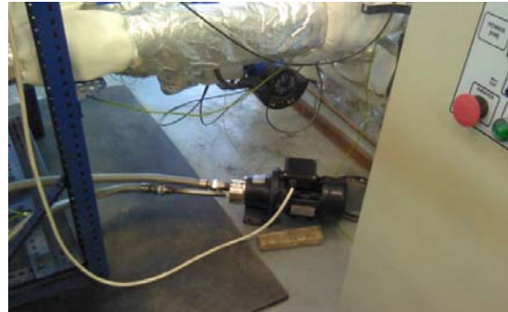
Fig. 6. The photo of the pump operating with the HFE7100
