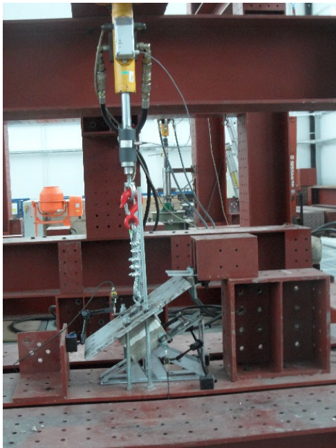
Fig. 7. Test stand during the examination of a single anchor test at an angle of 45° [9,10]
