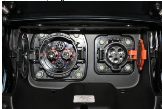
Fig.5 Nissan Leaf charging plugs, from left CHAdeMO and from right SAE J1772 type 1 (US) [6]
