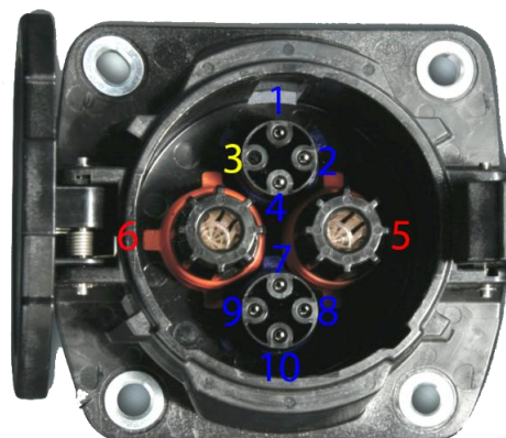
Fig.6 Zoom and description of CHAdeMO plug [6]
