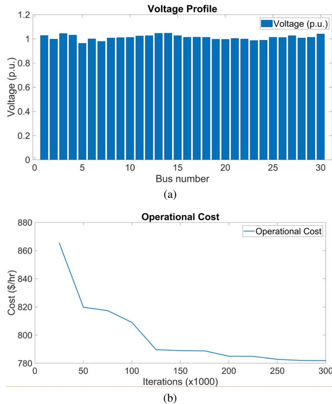
Fig. 2. Voltage profile (30 – bus) (a); cost minimization (30 – bus) (b)
