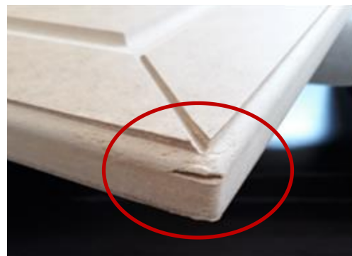
Fig. 2. An example of mechanical damage to the furniture front.
