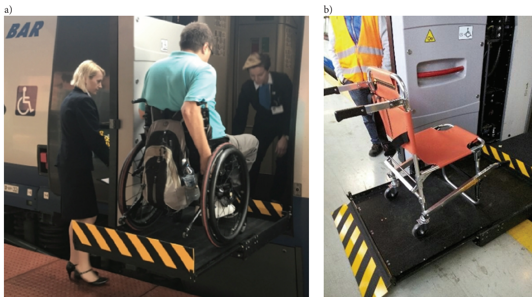
Fig. 16. Lift mounted near the coach doors: a) while lifting a traveller on a wheelchair [22], b) chair on a lift for persons with reduced mobility who do not use wheelchairs [23]
