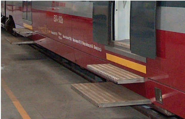
Fig. 19. Vehicle type ED74 with propounded steps [29]
