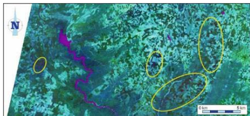
Fig. 6. ETM+ band ratios 3/5, 4/1 and 5/7 as RGB, respectively. The presence of iron oxides corresponds to the violet zones in the ellipses
