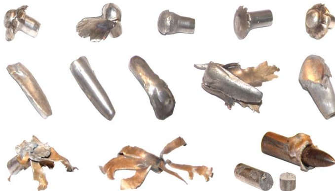
Picture 5. Fragments of regular bullets LPS (cartridge 7.62x54R mm) and PS (cartridge 7.62x39 mm) damaged at ricocheting against steel obstacle and armour piercing-incendary bullet B-32 and its core broken at ricocheting (bottom right) [1]
