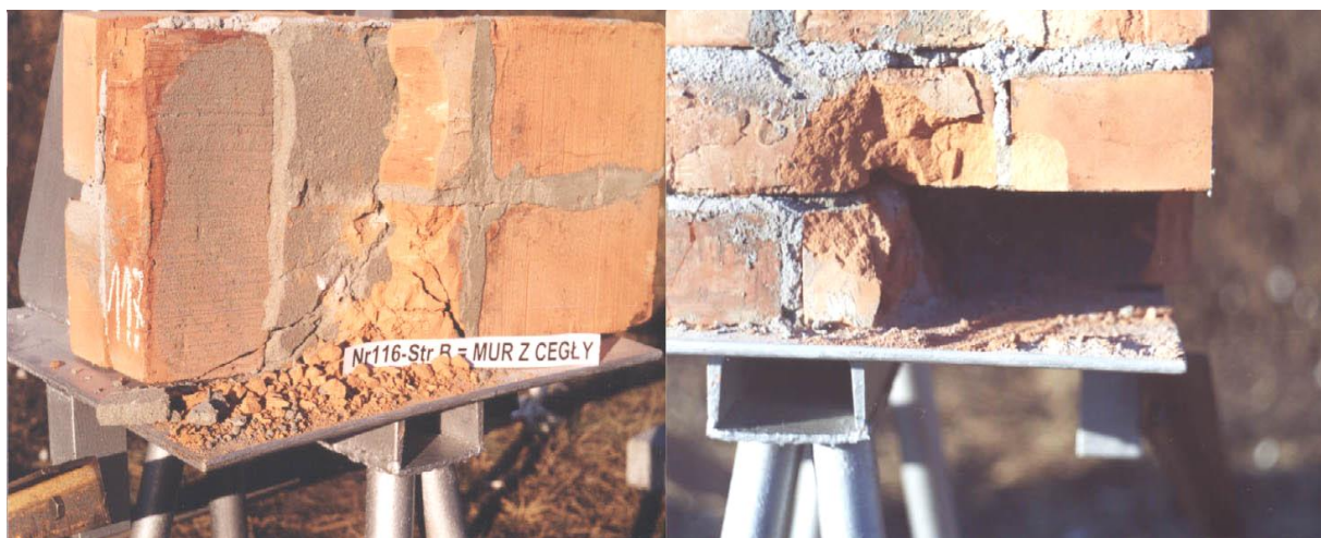
Picture 1. Results of bullet hitting at a wall of bricks [4]
