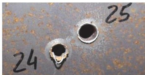
Picture 3. Results of hitting into steel plate St3S with thickness 8 mm: service regular round 7.62x51 mm (trace No 24) and round 7.62x51 mm of training ammunition (trace No 25) [4]
