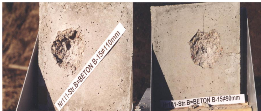
Picture 2. Views of outgoing craters on the testing samples made from B-15 class concrete [4]
