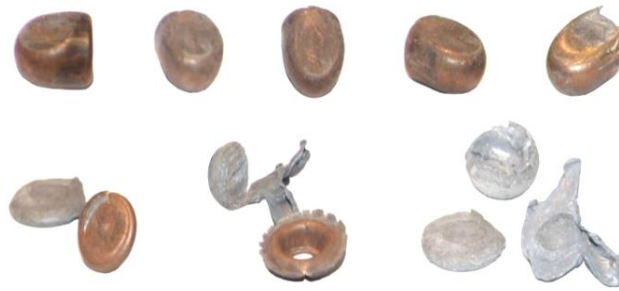
Picture 4. Bullets 9x18 mm of Makarow ammunition with different levels of deformation after ricocheting on the steel obstacle [1]
