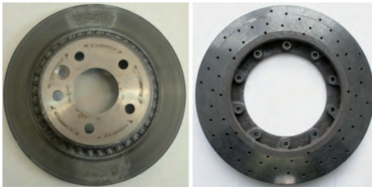
Fig. 1. Brake disc made of AIMC (a) and CF-C (b) after tribological tests
