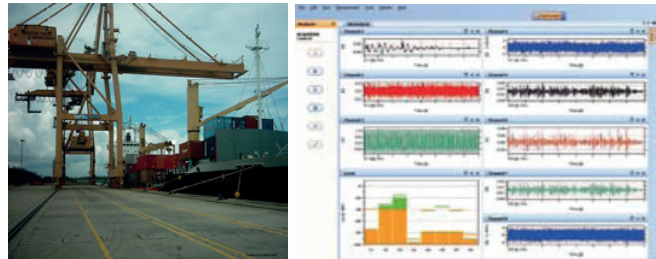
Fig.1. View of port crane and recording results of the dynamic state of using vibration
