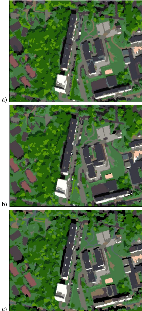
Fig. 4. Three results of object-based classification: a) in original image layers, b) after PCA and c) HCS/W sharpening transformation.
