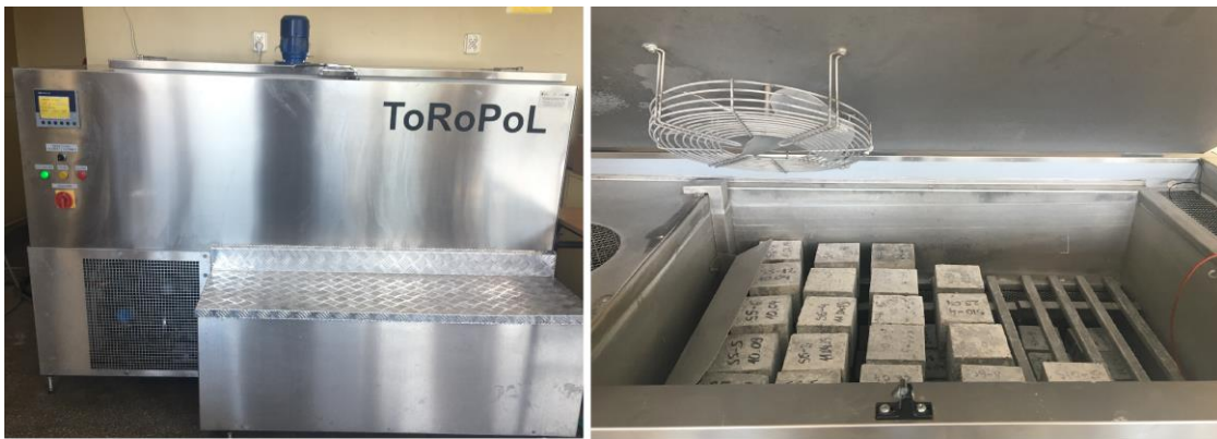
Figure 3. Device for testing frost resistance (own elaboration)
