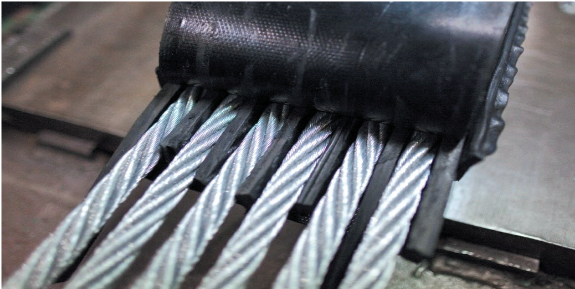
Fig. 2. SAG-type steel rubbercoated flat balance rope [2]
