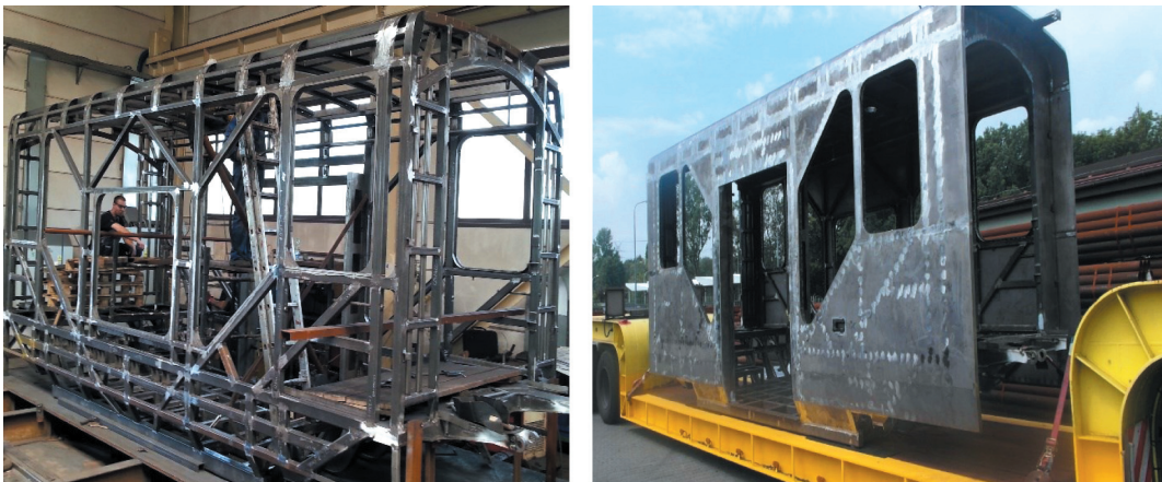
Fig. 5. Construction of the middle section of a tram car [3]
