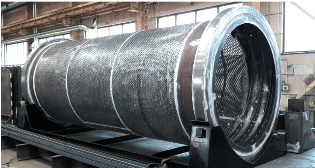
Fig. 6. Construction of a drum screen [3]
