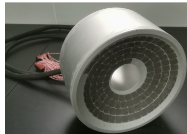
Fig. 2. Image of the as-fabricated 128-sector vortex Archimedean spiral phased array transducer.
