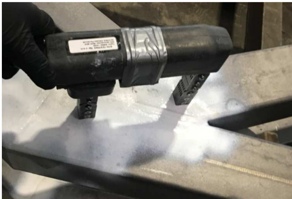
Fig. 4. Position of magnetic defectoscope during ultrasonic testing (UT) of brace to lower chord assembly splice
