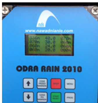
Figure 3. Values declared during tests – length and speed of rolling of the sprinkler hose
