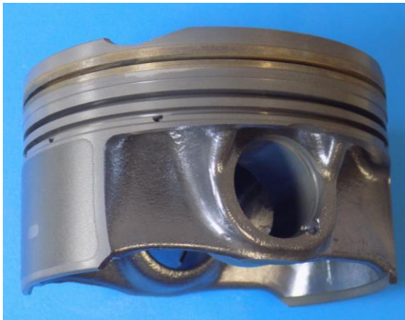
Fig. 1. Subject of tests - Diesel engine piston model
