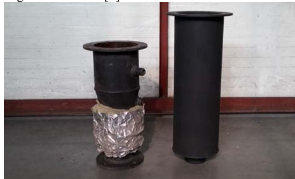
Fig. 12 The muffler (right) in comparison with rear cover of the heat exchanger (left)
