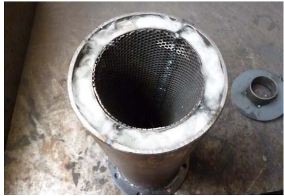
Fig. 11: Glass wool inside of muffler
