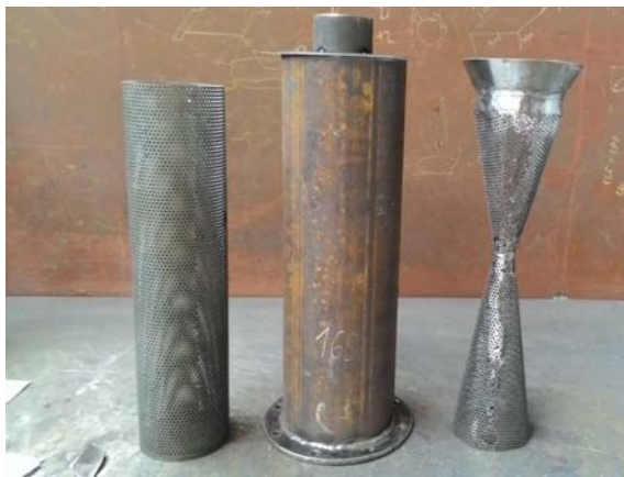
Fig. 10: Parts of muffler
