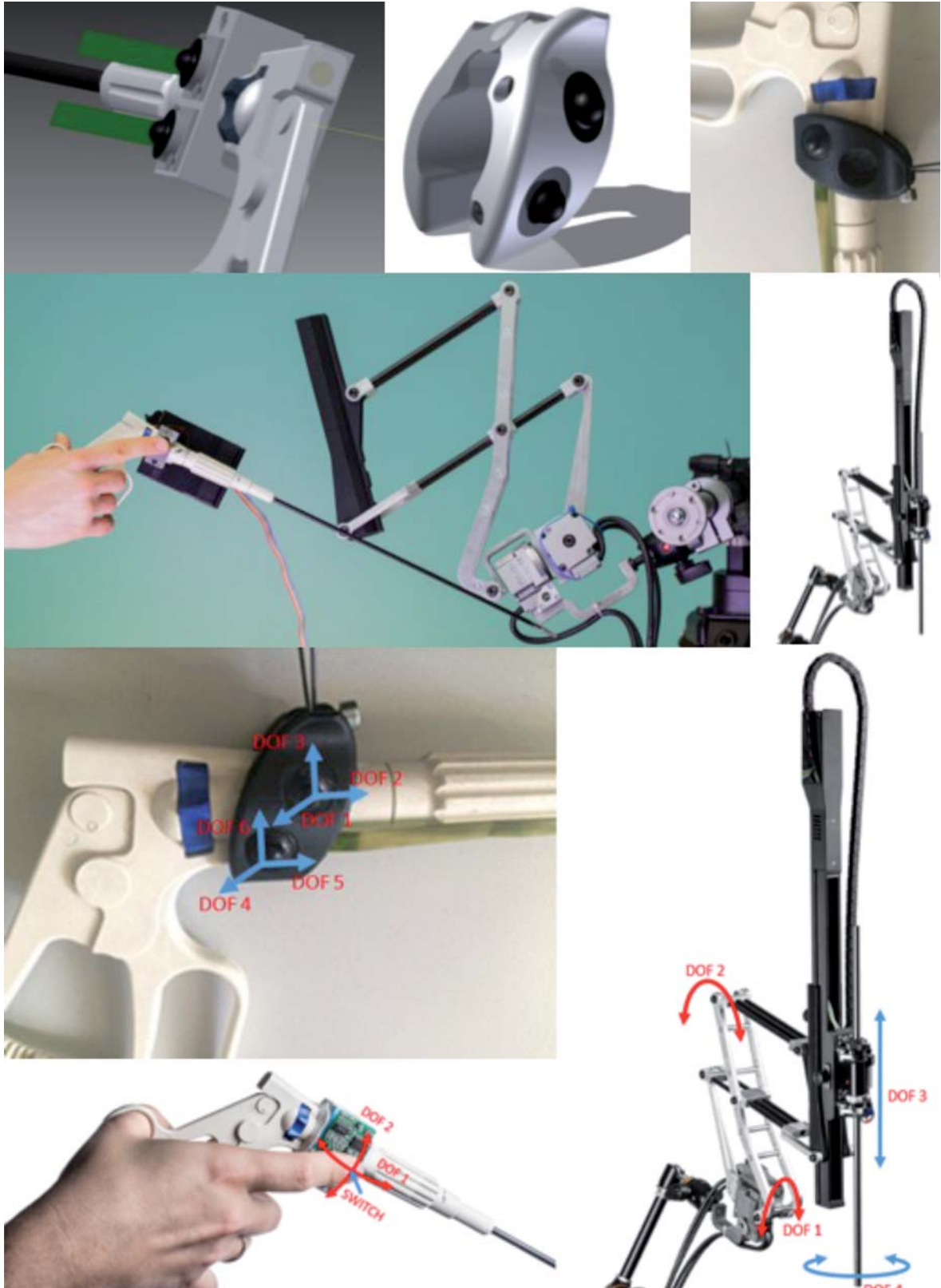
Figure 9. The assembly of the manufactured force sensors onto the endoscopic tools of Robin Heart Vision robot for controlling motion/position/orientation.
