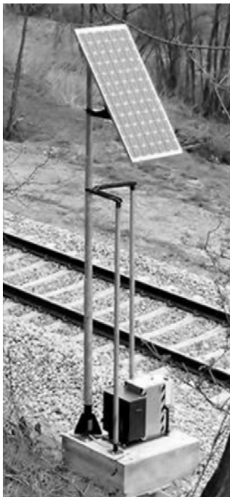
Fig. 4. CL-E1 device detects the train (a) and apply CHFC material with use of dosing element (b) directly to the desired location in the optimal concentration
