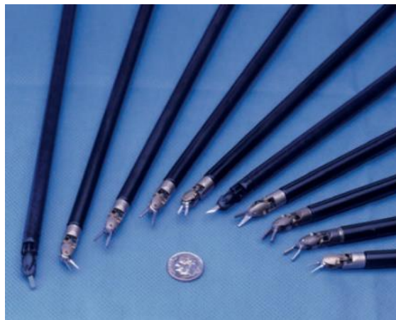
Figure 3. Examples of da Vinci robot work attachments [2]
