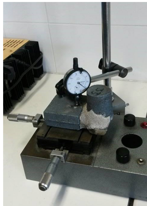
Fig. 8. Measuring tool for cerioxide depth
