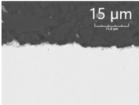
Fig. 2. Cross-section view outside ceroxide zone (SEM – BSE)
