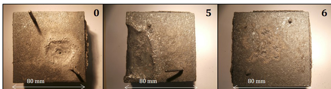
Fig. 11. Influence of different coatings on ceroxide formation
