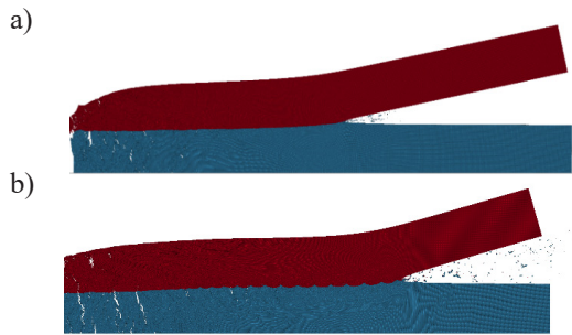
Fig. 4. Comparison of results obtained from the simulations with 2000 m/s initial velocity of the flyer plate for 12-degree (a) and 16-degree (b) initial impact angles
