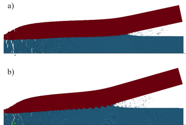
Fig. 6. Comparison of results from the model with 2500 m/s initial velocity of the flyer plate: 12-degree (a) and 16-degree (b) initial impact angles
