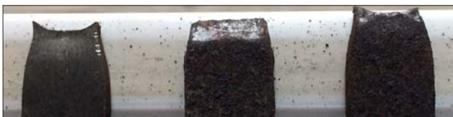
Fig. 11. Fracture of the tensile test pieces
