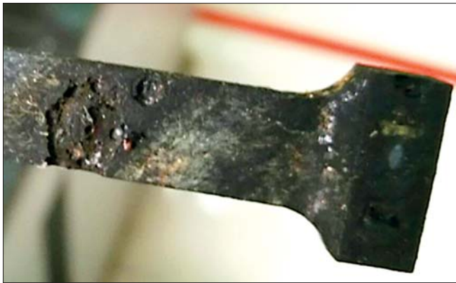
Fig. 5. Severely corroded test piece
