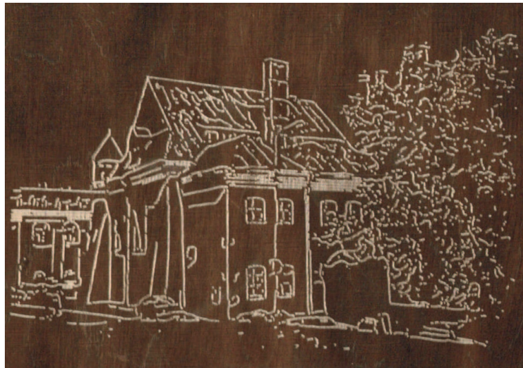
Figure 15. Drawing made in wood with CNC milling machines
