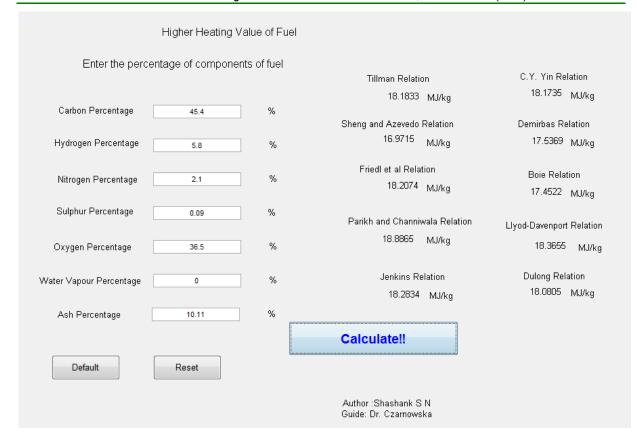
Fig 3.1 MATLAB application developed for the HHV calculation
