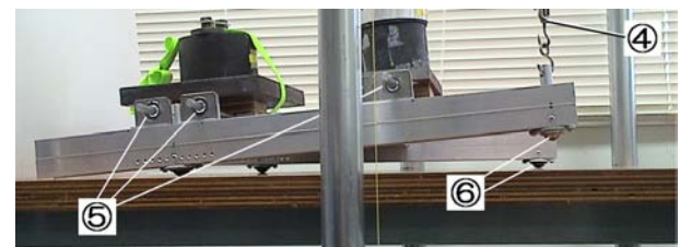
Fig. 10. Overview of the experimental setup that measures flexure while changing the lift force at the right rear of the chassis. Circled numbers from 1 to 6 refer to dummy weight, electric spring gauge, height gauge, turnbuckle, spherical joint, and spherical caster, respectively
