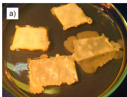
Figure 1. Method of agar flooding. Growth of: a) bacteria on box pad for confectionary, b) board box.
