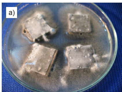
Figure 2. Agar flooding method. Growth of mould on: a) pizza packaging, b) paperboard samples, c) box paperboard.
