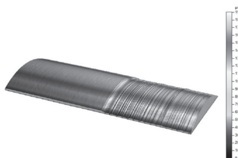
Fig. 4. Stereometric image of the area of the transition zone between the non-friction and the friction area – disc burnished surface ( R_k = 10\ \text{mm} , f = 0.255\ \text{mm/rev.} , F = 2.75\ \text{kN} ) after wearing on a distance of 9,500 m
