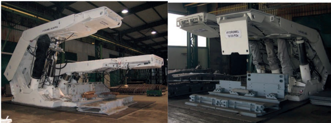
Fig. 1. HYDROMEL-16/34-POz and 16/35-POz powered roof support [3]
