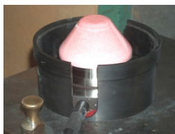
Figure 12. Pressed shaped piece in the female mould ‘take up’.
