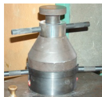
Figure 11. Mould 1 prepared for ejecting of the shaped piece.
