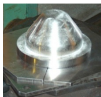
Figure 7. Base of mould 1 with the ‘distance forks’ on the press cart.
