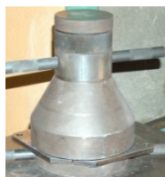
Figure 10. Mould 1 after pressing of the shaped piece.
