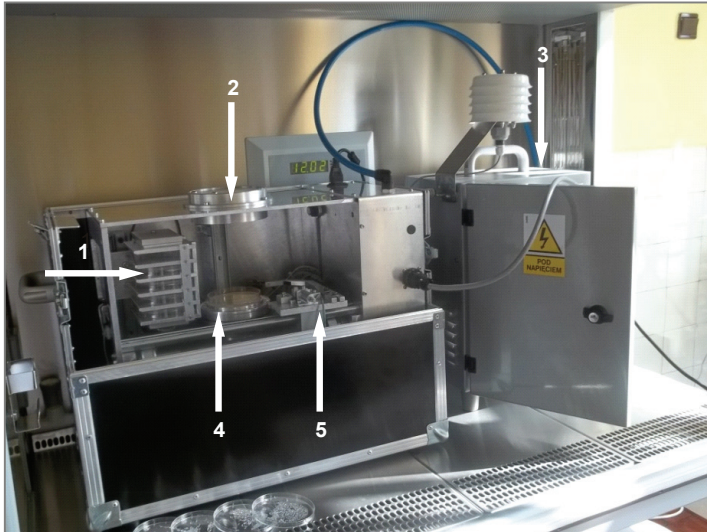
Fig. 1. Testing version (not final) of a new bioaerosol sampler with a split impactor: 1 – store box of Petri dishes, 2 – top of the impactor with 100 round nozzles, 3 – pump, 4 – bottom of the impactor, 5 – installation for transportation of Petri dishes (Patent pending: No.: WIPO ST 10/C PL400378)
