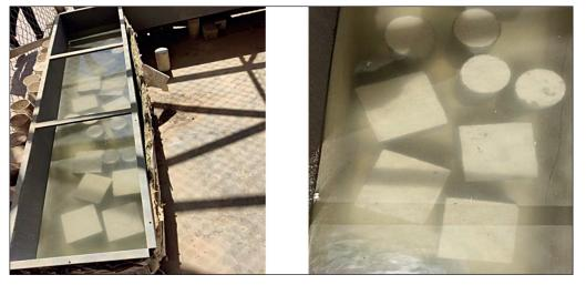
Figure 6. Curing process
