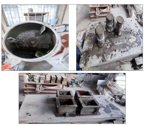
Figure 5. Mixing and casting of concrete
