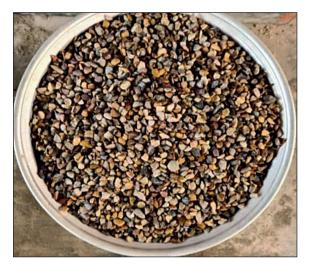
Figure 2. Natural coarse aggregate
