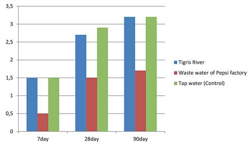
Figure 10. Graph of splitting tensile strength against age of concrete
