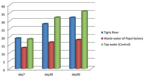
Figure 9. Graph of compressive strength against age of concrete
