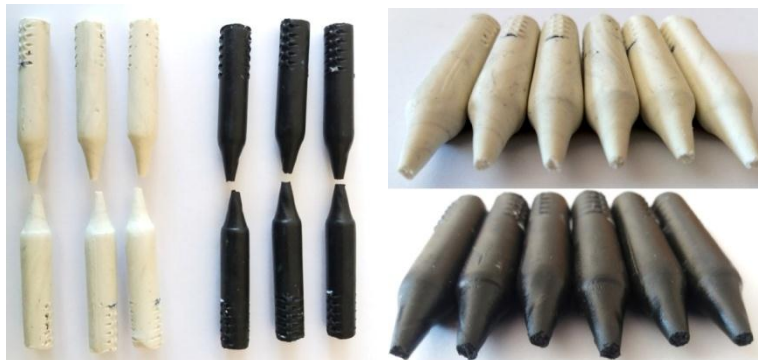
Fig. 5. Slip of the charge due to tensile test
