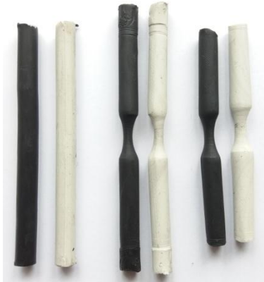
Fig. 3. The order of sample preparation (starting from the left: bar extrusion, narrowing of the bar, cutting of the sample to the length)
