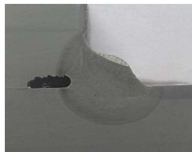
Fig. 4. Pictures illustrating results of the macroscopic testing of S460N steel; a) the specimen W3.1: cracks along fusion line and in HAZ; b) the specimen P5.1: no imperfections. Etching: Nital
