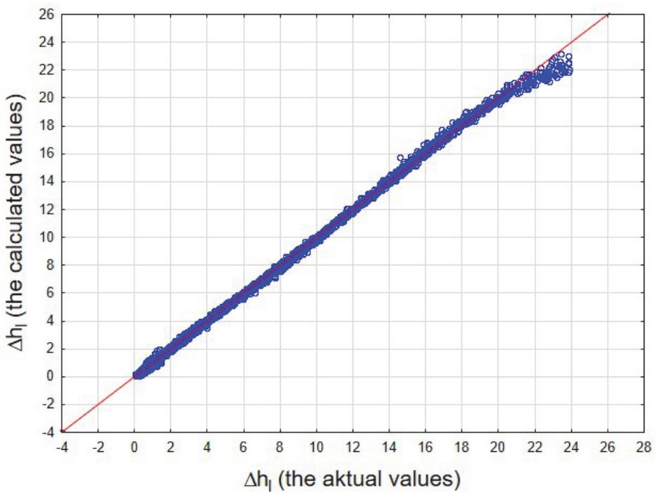
**Fig. 2.** The relationship between the actual values of pressure losses  $\Delta h_l$  and those calculated by the artificial neural network
